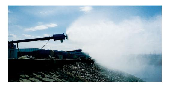
ParKwater® HV15B is a land-based mechanical vaporizer. It is simply designed, stable and reliable. Best for larger areas where wastewater contains lower dissolved solids or smaller to no particulates. It is a better solution to wastewater.
